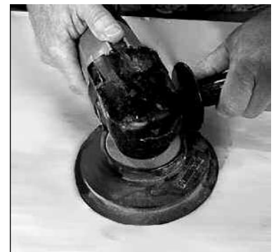
Fig. 18 Sanding using random Orbital sander
