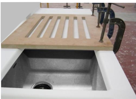
Fig. 11 Drainer Groove Jig clamped in position and ready to be routed.
