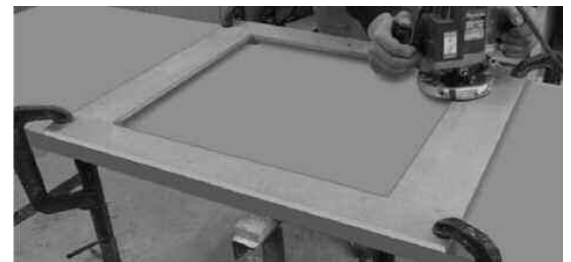
Fig. 9 Hob/Sink template clamped in position
